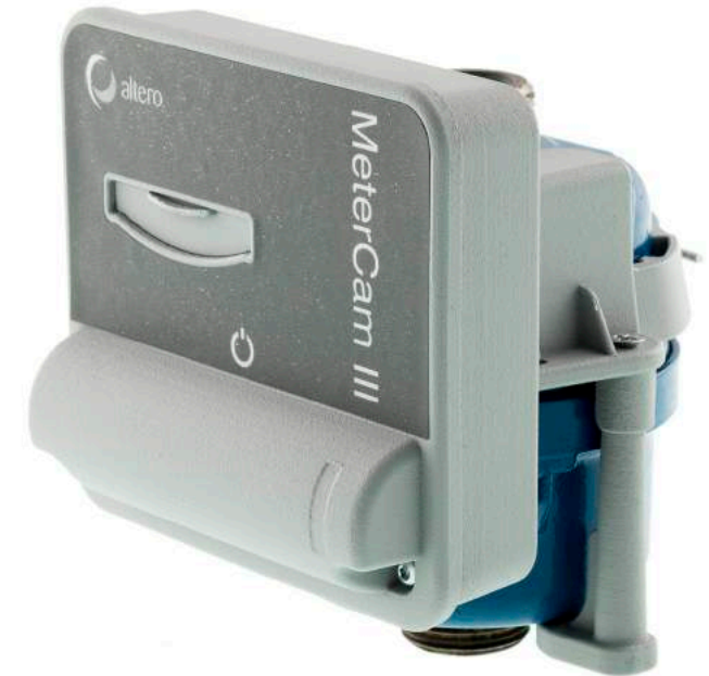
The MeterCam installed on a water meter.
