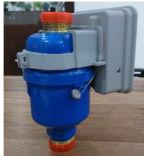
A MeterCam installed on a water meter.
