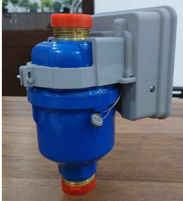
The MeterCam installed on a water meter.
